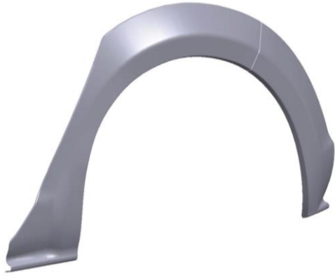
Three-dimensional illustrative view of a fender flare for the left rear wheel well of a vehicle
