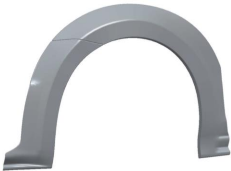
Three-dimensional illustrative view of a fender flare for the left front wheel well of a vehicle
