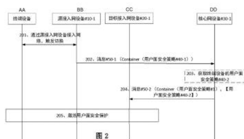
201 Access a network by means of the source access network device, so as to trigger switching 202 Message #50-1 (Container (user plane security policy #40-1)) 203 Acquire a user plane security policy #40-2 of the terminal device 204 Message #50-2 (Container (user plane security policy #1), (user plane security policy #40-2)) 205 Activate user plane security protection AA: Terminal device BB: Source access network device #10-1 CC: Target access network device #20-1 DD: Core network device #30-1
